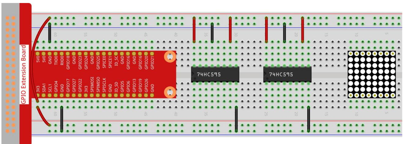
**Step 2:** Connect pin 11 of the two 74HC595 together, and then to GPIO27; then pin 12 of the two chips, and to GPIO18; next, pin 14 of the 74HC595 on the left side to GPIO17 and pin 9 to pin 14 of the second 74HC595.
