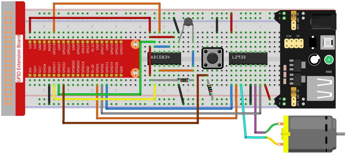
**Note:** The power module can apply a 9V battery with the 9V Battery Buckle in the kit. Insert the jumper cap of the power module into the 5V bus strips of the breadboard.
