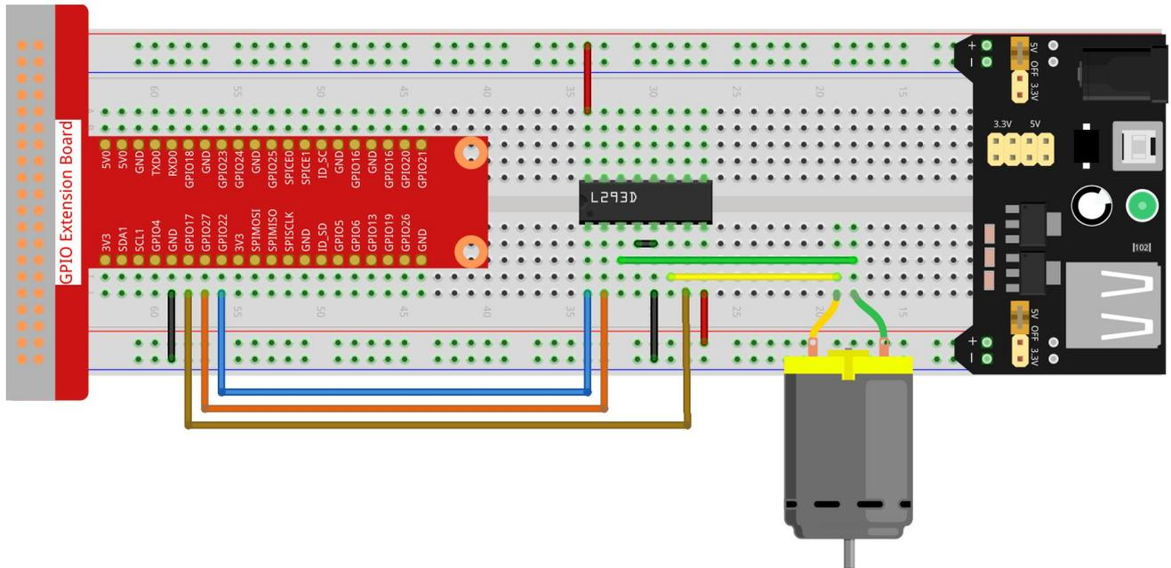
**Note:** The power module can apply a 9V battery with the 9V Battery Buckle in the kit. Insert the jumper cap of the power module into the 5V bus strips of the breadboard.
