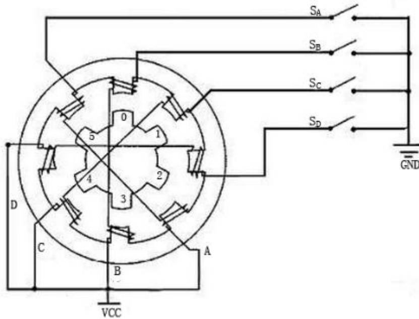
The four-phase stepper motor has three operating modes: single four-step, double four-step, and eight-step. The step angle for the single four-step and double four-step are the same, but the driving torque for the single four-step is smaller. The step angle of the eight-step is half that of the single four-step and double four-step. Thus, the eight-step operating mode can keep high driving torque and improve control accuracy.
