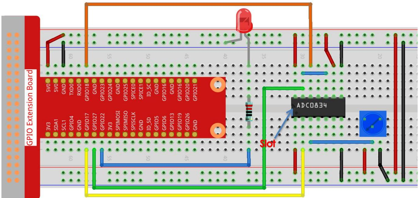
Note: Please place the chip by referring to the corresponding position depicted in the picture. Note that the grooves on the chip should be on the left when it is placed.
