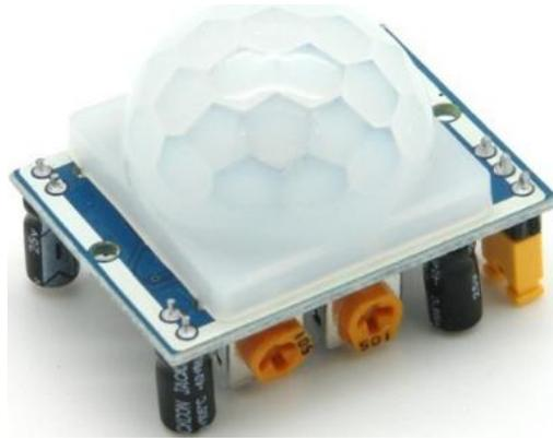
After the sensing module is wired, there is a one-minute initialization. During the initialization, module will output for 0~3 times at intervals. Then the module will be in the standby mode. Please keep the interference of light source and other sources away from the surface of the module so as to avoid the misoperation caused by the interfering signal. Even you'd better use the module without too much wind, because the wind can also interfere with the sensor.
