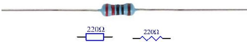
When using a resistor, we need to know its resistance first. Here are two methods: you can observe the bands on the resistor, or use a multimeter to measure the resistance. You are recommended to use the first method as it is more convenient and faster. To measure the value, use multimeter.
