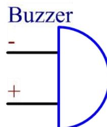
You can check the pins of the buzzer, the longer one is the anode and the shorter one is the cathode. Please don't mix them up when connecting, otherwise the buzzer will not make sound.
