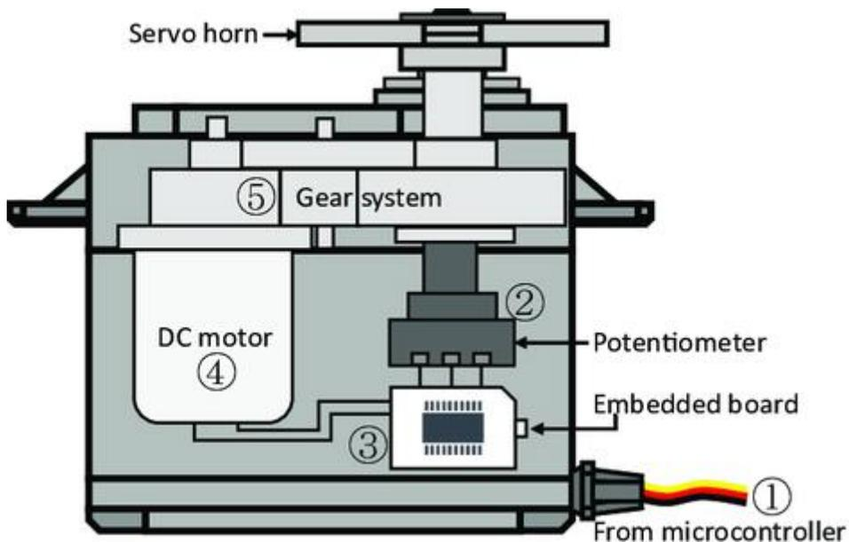
The angle is determined by the duration of a pulse that is applied to the control wire. This is called Pulse width Modulation. The servo expects to see a pulse every 20 ms.
