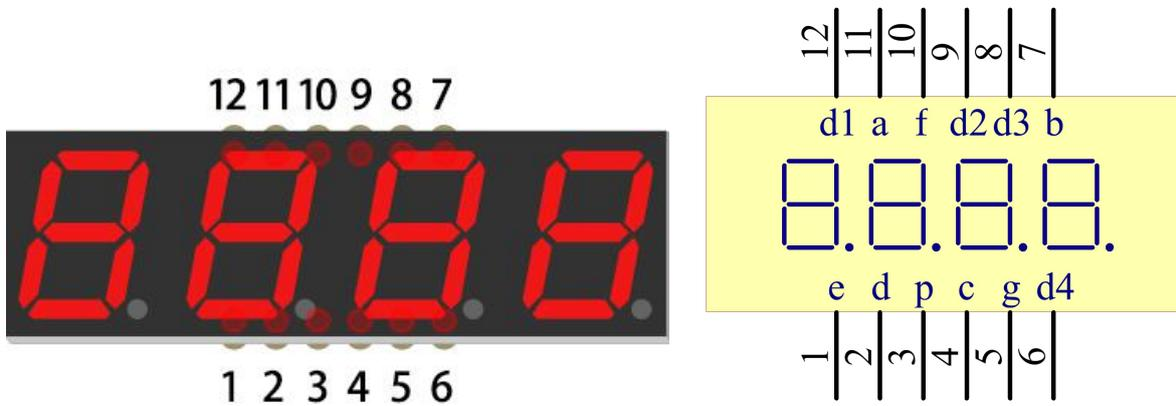
The 4-digital 7-segment display works independently. It uses the principle of human visual persistence to quickly display the characters of each 7-segment in a loop to form continuous strings.
