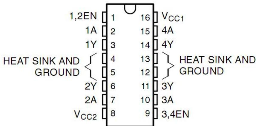
The following is the internal structure of L293D. Pin EN is an enable pin and only works with high level; A stands for input and Y for output. You can see the relationship among them at the right bottom. When pin EN is High level, if A is High, Y outputs high level; if A is Low, Y outputs Low level. When pin EN is Low level, the L293D does not work.
