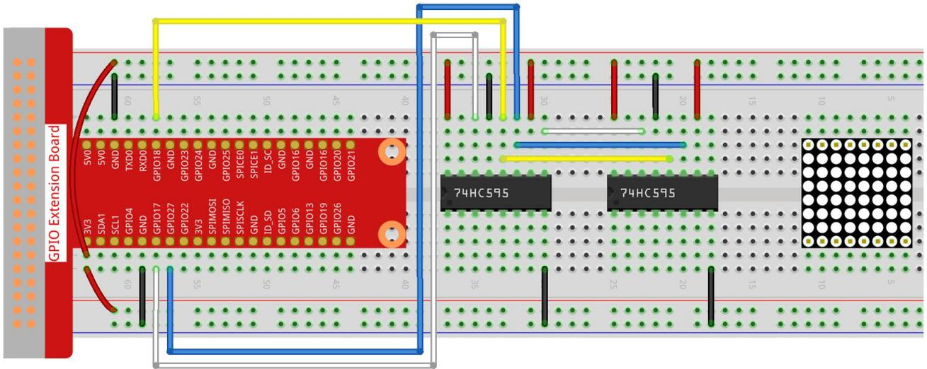
**Step 3:** The 74HC595 on the right side is to control columns of the LED dot matrix. See the table below for the mapping. Therefore, Q0-Q7 pins of the 74HC595 are mapped with pin 13, 3, 4, 10, 6, 11, 15, and 16 respectively.
