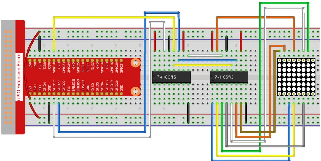
**Step 4:** Now connect the ROWs of the LED dot matrix. The 74HC595 on the left controls ROW of the LED dot matrix. See the table below for the mapping. We can see, Q0-Q7 of the 74HC595 on the left are mapped with pin 9, 14, 8, 12, 1, 7, 2, and 5 respectively.
