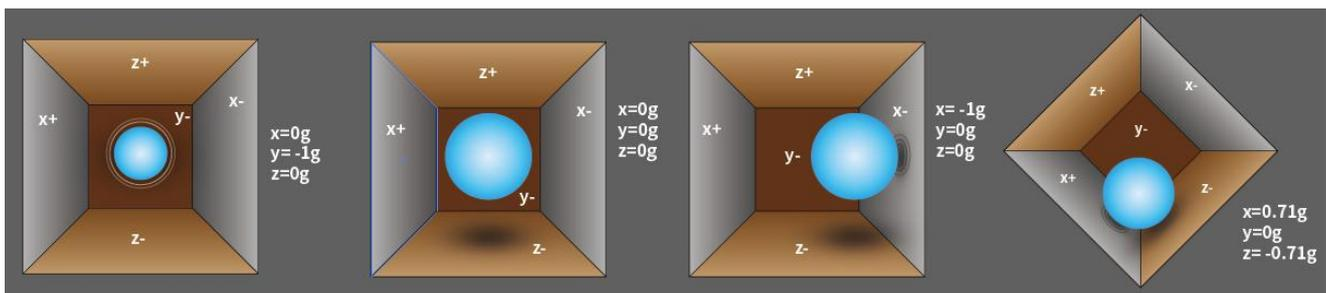
We can use the MPU6050 to detect its acceleration on each coordinate axis (in the stationary desktop state, the Z-axis acceleration is 1 gravity unit, and the X and Y axes
