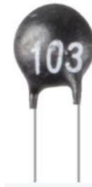
The principle is that the resistance of the NTC thermistor changes with the temperature of the outer environment. It detects the real-time temperature of the environment. When the temperature gets higher, the resistance of the thermistor decreases. Then the voltage data is converted to digital quantities by the A/D adapter. The temperature in Celsius or Fahrenheit is output via programming.
