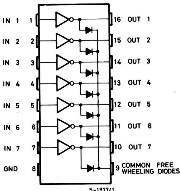
To apply the motor in the circuit, a driver board needs to be used. Stepper Motor Driver-ULN2003 is a 7-channel inverter circuit. That is, when the input pin is at high level, the output pin of ULN2003 is at low level, and vice versa. If we supply high level to IN1, and low level to IN2, IN3 and IN4, then the output end OUT1 is at low level, and all the other output ends are at high level.
