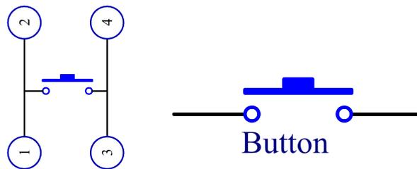
When the button is pressed, the 4 pins are connected, thus closing the circuit.
