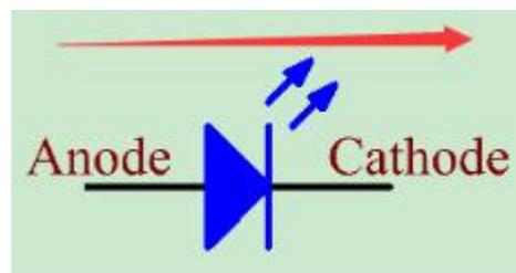
The LED can not be directly connected to power supply, which can damage component. A resistor with 160Ω or larger (work in 5V) must be connected in series in the circuit of LED.
