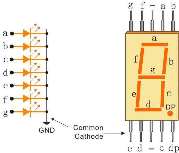
Each of the LEDs in the display is given a positional segment with one of its connection pins led out from the rectangular plastic package. These LED pins are labeled from "a" through to "g" representing each individual LED. The other LED pins are connected together forming a common pin. So by forward biasing the appropriate pins of the LED segments in a particular order, some segments will brighten and others stay dim, thus showing the corresponding character on the display.
