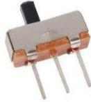
A slide switch, just as its name implies, is to slide the switch bar to connect or break the circuit, and further switch circuits. The common-used types are SPDT, SPTT, DPDT, DPDTT etc. The slide switch is commonly used in low-voltage circuit. It has the features of flexibility and stability, and applies in electric instruments and electric toys widely.
