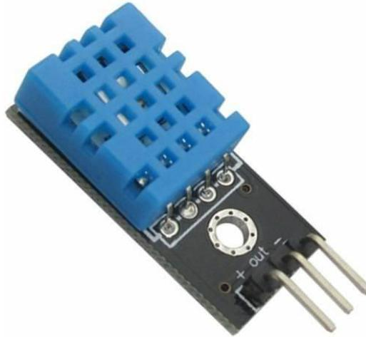
Only three pins are available: VCC, GND, and DATA. The communication process begins with the DATA line sending start signals to DHT11, and DHT11 receives the signals and returns an answer signal. Then the host receives the answer signal and begins to receive 40-bit humiture data (8-bit humidity integer + 8-bit humidity decimal + 8-bit temperature integer + 8-bit temperature decimal + 8-bit checksum). For more information, please refer to DHT11 datasheet.
