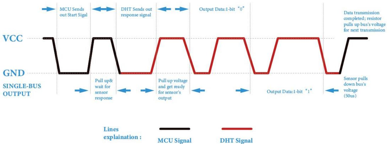
When DHT11 starts up, MCU will send a low level signal and then keep the signal at high level for 40µs. After that, the detection of the condition of external environment will start.
